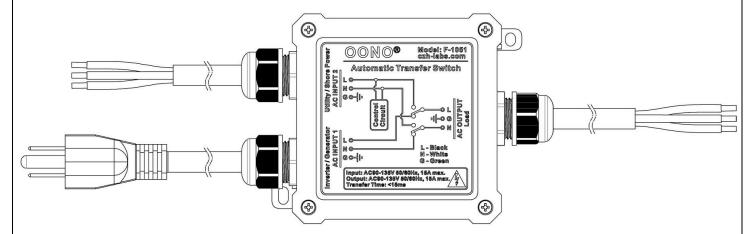
AC INPUT 1: US standard NEMA 5-15P 3 prong plug. Recommended connect Inverter or Generator.
